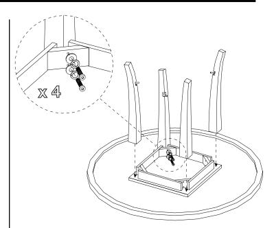
(3) With the assistance of another adult, carefully place tabletop upside side down onto a clean, padded surface. Insert 4 legs into tabletop as shown. Very loosely attach each leg with 2 bolts, 2 spring washers, and 2 flat washers.
