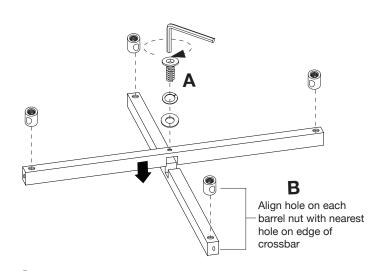
(1) A) Fit top crossbar onto bottom crossbar as shown. Secure crossbars with 1 small bolt, 1 spring washer, and 1 flat washer using an allen wrench. B) Remove small screws from each barrel nut and set aside. Insert 4 barrel nuts into crossbar assembly as shown. With a flat head screwdriver, align hole on each barrel nut with nearest hole on edge of crossbar assembly.
