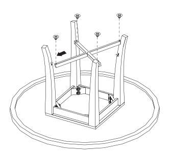
(4) Fit holes of crossbar assembly into barrel screws of each leg assembly as shown. Make sure each barrel nut is aligned vertically with barrel screw. Secure crossbar with 4 screws from step 1B using a screwdriver. Tighten the 8 leg bolts securely. With the assistance of another adult, position unit upright.
