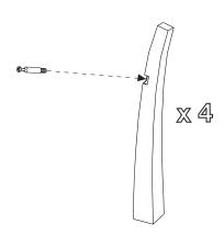
(2) Insert 1 barrel screw into each leg as shown. Secure screws with a phillips head screwdriver.
