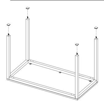
4 Insert 1 **tube cap** into the open end of each leg. If necessary, gently tap each tube cap into position with a **hammer**.
