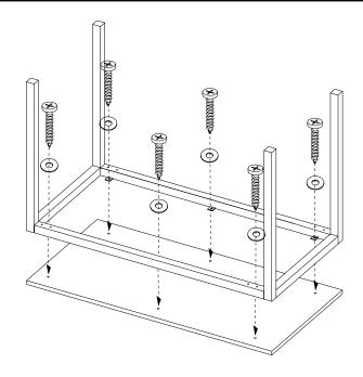
3 Position frame assembly onto table top, aligning holes in tabs with pre-drilled holes in table top. Using a **phillips** head screwdriver, secure each tab with 1 wood screw and 1 washer.
