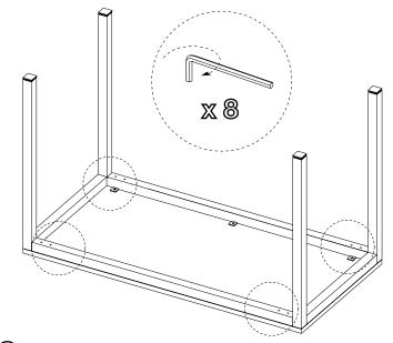
(5) At this point, fully tighten all 8 allen head screws with the allen wrench.
