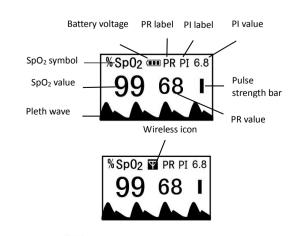
Icon : indicates the wireless connection is set up between the mobile device and oximeter.
