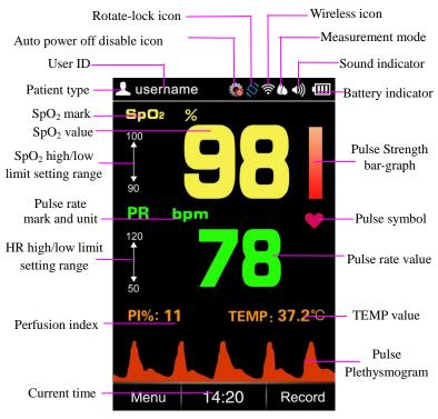
Figure 4.2A Default Display Screen---in vertical
