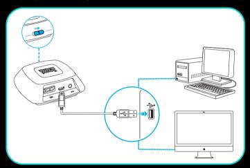
**NOTE** • Slide the Console/PC Mode switch on the transmitter to PC.
