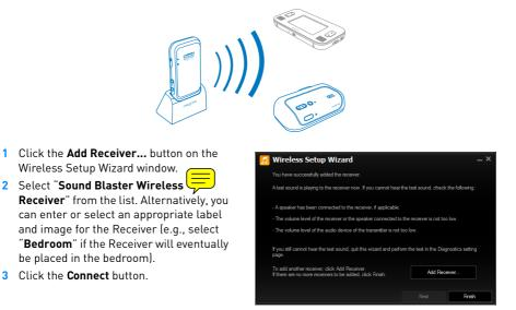
4 Turn on your Receiver and the attached speakers. Press the Connect button at the back of the receiver. Once the Transmitter and Receiver are paired successfully, the Connect LED lights up green and remain on. You should also hear a test tone played through the speakers that are attached to the Receiver.
