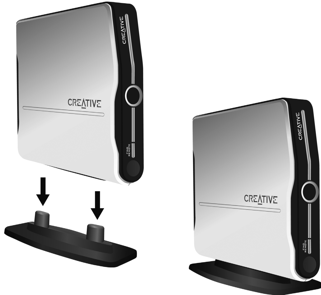
Figure 2-2: Attaching the stand to your Wireless Receiver (optional)
