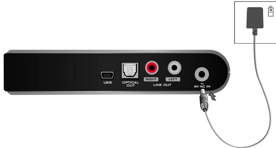
Figure 3-8: Connecting your Wireless Receiver to a power outlet
