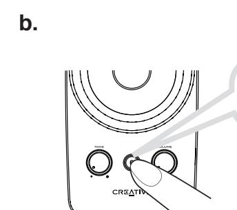
Press and Hold the CONNECT button for 3 sec, then release when 2 beep tones are heard with the LED Status Indicator blinking rapidly
