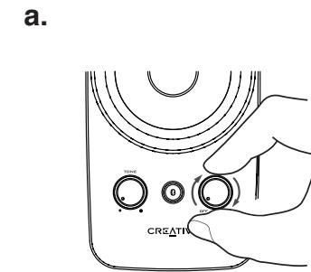
Power on the speaker by turning the knob in the clockwise direction and the LED Status Indicator will show blue. This indicates that upon power up, the status of the speaker is not connected to any devices.
