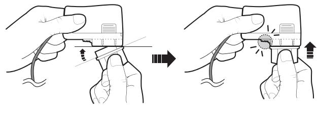
If you need to remove the plug head from the power adapter base, pull the latch to release the plug head, and gently remove it from the base.
