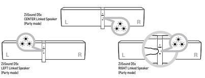
Press and hold the LINK TouchPad / Button for 4 seconds and release on the RIGHT Master speaker. Now all LED on the LINK LED status indicator will disappear, only displaying their respective Channel LED indicator indicating they are in MULTI-CHANNEL mode.
