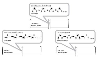
© LEFT and CENTER speakers are Linked when the LINK LED Status indicator of the LEFT and CENTER channel speakers shows their respective LEFT and CENTER LED Lit on its LINK LED.
