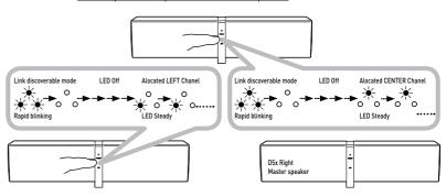
B Press and hold the LINK Touchpad / Button for 4 seconds until its LINK LEDs are rapidly blinking on the other ZiiSound D5x [s] speakers one after the other. They will be automatically be allocated as LEFT, then CENTER Channels by order of the activation of their LINK discovery mode. ie 2<sup>nd</sup> speaker to activate LINK discovery would be the LEFT Channel. 3<sup>nd</sup> speaker would be the CENTER Channel.
