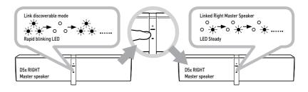
E Link establishment complete. If the ZiiSound D5x (Right Channel) Master speaker LINK LED is still Rapidly Blinking, Press the LINK Touchpad / Button once to stop or wait for it to timeout. The speakers are now in Multi Channel mode. Ready to Stream music.
