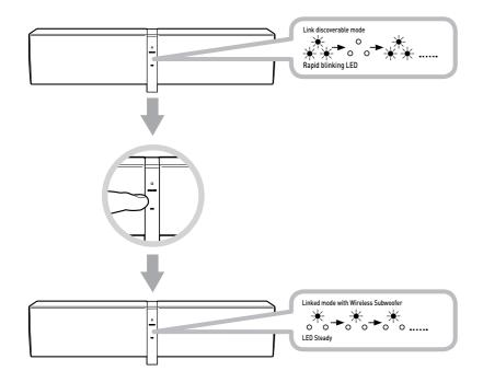
Link establishment complete. If the ZiiSound D5x LINK LED is still Rapidly Blinking, Press the LINK Touchpad / Button once to stop or wait for it to timeout. Ready to Stream music.
