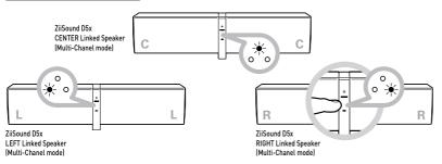
Press and hold the LINK TouchPad / Button for 4 seconds and release on the RIGHT Master speaker. Now all LED on the LINK LED status indicator will light up, indicating they are in PARTY mode configuration.
