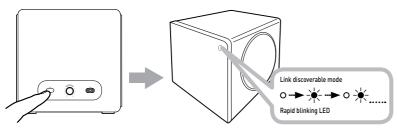
With the Subwoofer mains powered ON, press and hold the Link button for 4 Seconds until the LED is blinking rapidly. Subwoofer is now ready to receive connection from a master speaker unit.
