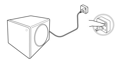
Plug in the AC cord into the AC IN and switch on the mains. The ZiiSound DSx is powered ON and in standby mode.
