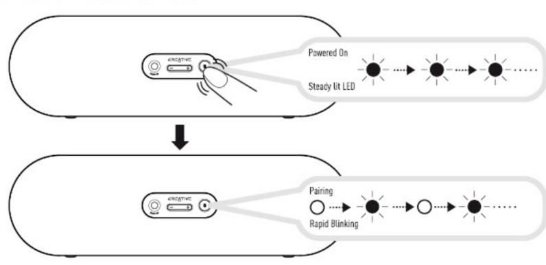
The LED status indicator will lit steady indicating the speaker is currently ON. To allow pairing to other Bluetooth devices, Press and Hold the CONNECT button for 3 seconds. Release when 2 beep tones are heard with the LED status indicator blinking rapidly.
