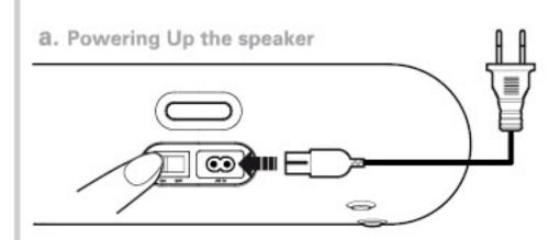
Attach the AC cord to the AC IN and flick the Power switch to ON position.
