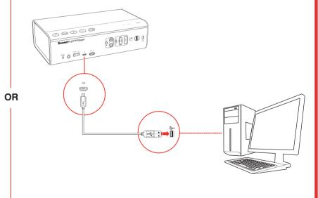
\* The speaker automatically goes into MicroSD Card Reader Mode every time it is connected to a computer. To use it for audio playback, see "Playing audio from computer (USB audio)".
