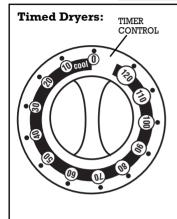
Select the required Drying time by rotating the Timer control clockwise (up to 120 minutes) just past the required time, then anti-clockwise to the desired time. Refer to the Drying guide.
