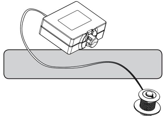
Blue LED is Inside the Relay Box, Light will Shine Through at the LED Placement Shown Below.
