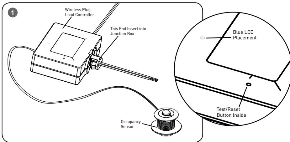
Blue LED is Inside the Relay Box, Light will Shine Through at the LED Placement Shown Below.
