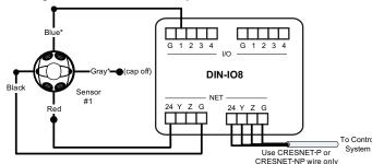
\*\*The following Crestron devices may be used to integrate the sensors into a Cresnet system by following the schematic shown here:
