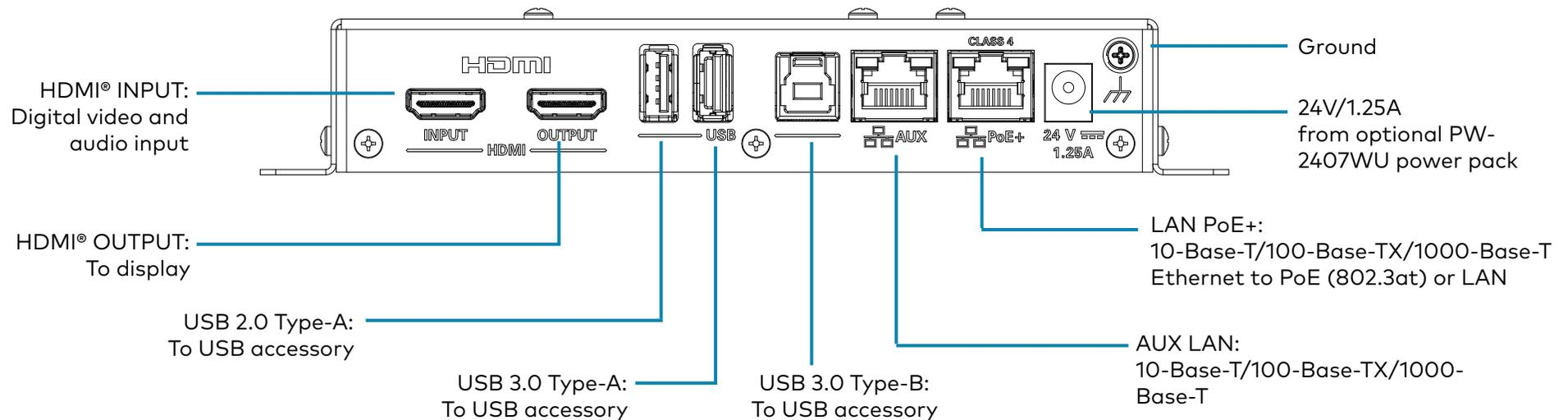
**NOTE:** PoE-type networks connected to these ports are for intrabuilding use only and should not be connected to lines that run outside of the building where this product is located.
