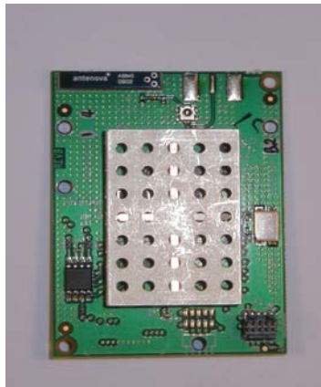
Physical View of CWD6782 (SMD antenna)
