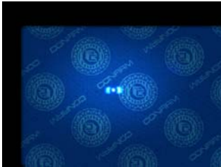
Image captured with an D SCAN AUTHENTICATOR CF under coaxial light showing a document having a 3M™ Confirm™ Laminate on top of the personalized page. The retro reflective marks are clearly visible while the underlying text and pictures are almost invisible.
