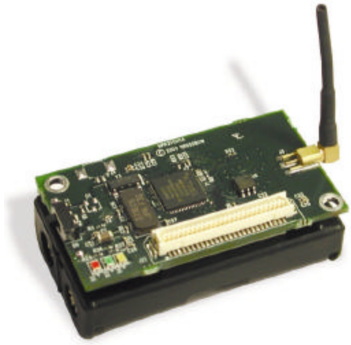
Figure 2-1. Photo of the MPR2400—MICAz with standard antenna. For the dimensions of the board and locations of the mounting holes, see Figure 2-2.
