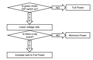
Figure 9.2.1 How Green Power DIP switches work
