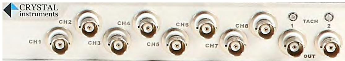
**Figure 21: Spider-80X Input Channels**
