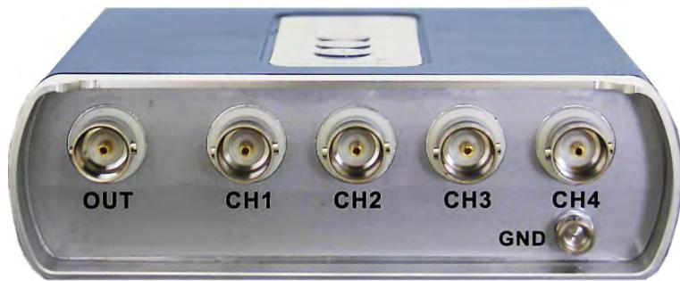
**Figure 20. Spider-20 Input Channels**
