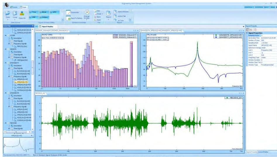
**Figure 143 Octave Spectra and FFT APS Processed at same time**
