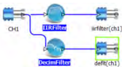
Figure 172. Example computing high and low sampling rate with a decimation filter.
