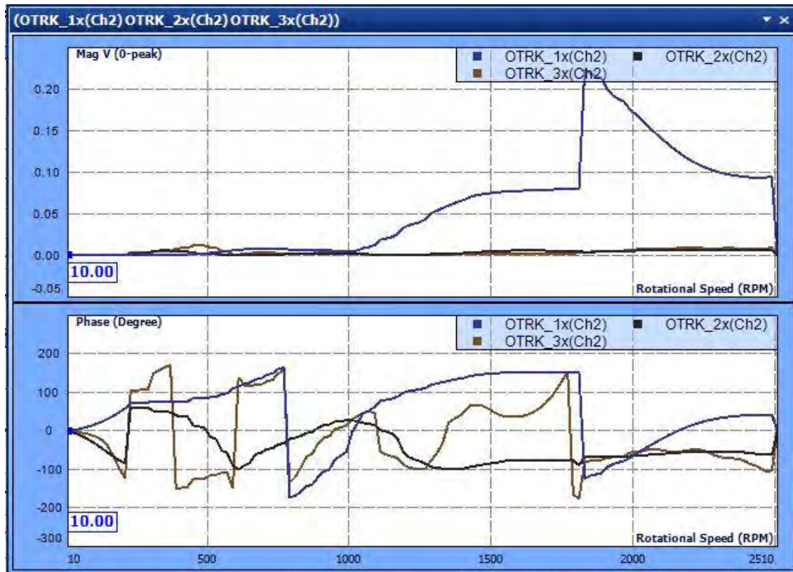
Figure 183: Typical Bode Plot
