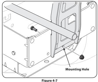
4. Secure the hanger assembly to the mounting assembly using a 5/16" bolt and flange nut provided. See Fig. 4-7.
