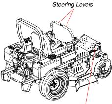
Figure. 3 Foot Pedal Lift
