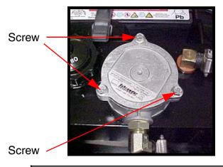
**Note:** Always wipe off the hydraulic tank fill cap and the area around it before removing the cap to prevent dirt from contaminating the oil.
