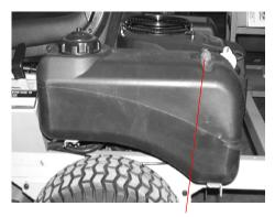
Figure. 4 Fuel Shutoff Valve
