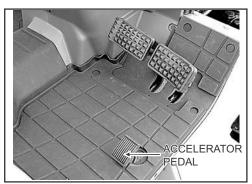
Use this pedal when operating the tractor on the road. Push the pedal down to increase engine speed.
