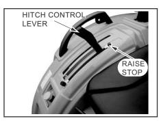
If raise stop setting position is incorrect, the hydraulic pump might be damaged. Therefore carefully adjust as below.
