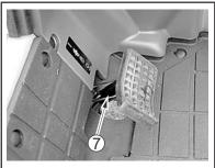
For long term storage, lock the clutch pedal in the disengaged position. This will prevent the clutch disc from sticking to the engine flywheel.
