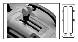
— Move the lever forward to engage the Mid PTO. Move the lever rearward to disengage the Mid PTO.
