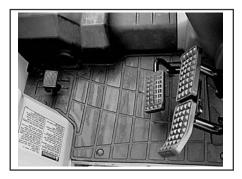
HST control pedal in the N position CLUTCH pedal (HST Drive)
