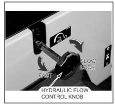
**NOTE:** When transporting the tractor on the road with the implement mounted on the three point hitch, always set flow control knob to the LOCK position.
