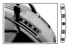
Move the range shift lever forward to place the transmission in H range.
