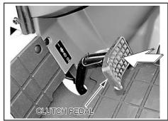
Push the clutch pedal down.
