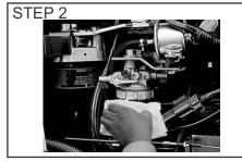
Clean the outside of the filter body and cup to prevent dirt or foreign materials from entering the system.
