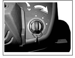
Turn the starter key switch to the heat & ON position.
