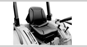
The seat is adjustable fore and aft by moving a lever.
