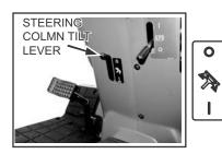
The steering wheel angle can be adjusted in three positions by the lever located under the steering column.
