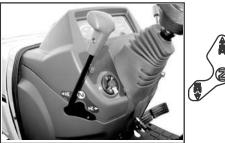
The shuttle shift lever is used to shift the transmission gear into forward of reverse position. Move the shuttle shift lever forward (F position) to the forward position. Move the shuttle shift lever rearward (R position) to the reverse position. The center position between F and R places the transmission in N position. (neutral)
