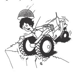
For towing, be sure to use the drawbar only. Set the hitch point below the center line of the rear axle. When using a chain, never try to move forward abruptly.
