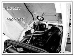
Lift the hood, and insert the Support Rod into hole. Remove both side covers.
