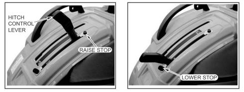
**IMPORTANT:** Position of the raise stop should not be set so rearward that insufficient free play of the lift arms is available at the highest position when hitch control lever is moved to the raise stop.
