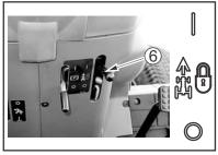
To keep a constant forward travel speed, move the lever fully upward, while holding the speed ratio control pedal at the desired speed. It does not work in reverse.
