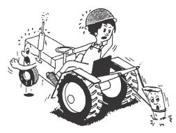
Avoid operating the tractor on an extreme slope that appears hazardous, when forced to operate on such slope, use extra care. Driving forward out of a ditch or mired condition or up a steep slope could cause tractor to tip over rearward.
