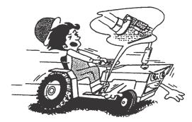
Never operate the differential lock while driving at high speed or traveling on the road. For driving the 4-WD tractor on the road, be sure to place the 4-WD shift lever in OFF position. C-4. Steering and Turning the Tractor
