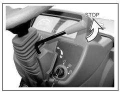
Move the engine speed control lever to run engine at idle speed for three to five minutes to decrease the temperature of engine.
