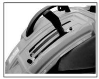
5. HITCH CONTROL LEVER — Use this lever to control the position of the hitch. Move the lever forward to lower the hitch to the required depth. Move the lever to the rear to raise the hitch to the required height.
