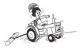
When operating the tractor on either a steep slope or flat ground, be sure not to suddenly steer, brake, clutch or operate attachments.
