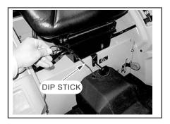
To check the transmission oil level, put the tractor on level ground.
