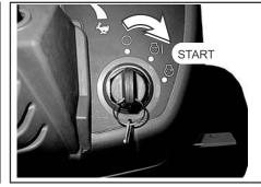
Turn key switch to start position until engine starts, but no more than 10 seconds, then release the key. Run engine for two minutes at 1500 RPM.
