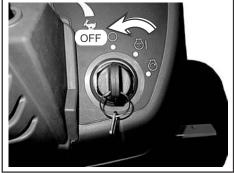
Turn the key switch to OFF position. Remove the key.
