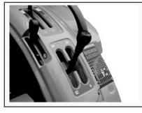
— The gear shift lever is used to shift the transmission gears into any of four speeds.
