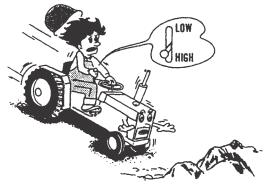
To start traveling, lower the engine speed and release the clutch pedal slowly. Before leaving the tractor, stop the engine, remove the key, apply the parking brake and make sure that the engine has come to a complete stop, and any attachment is completely touching the ground.
