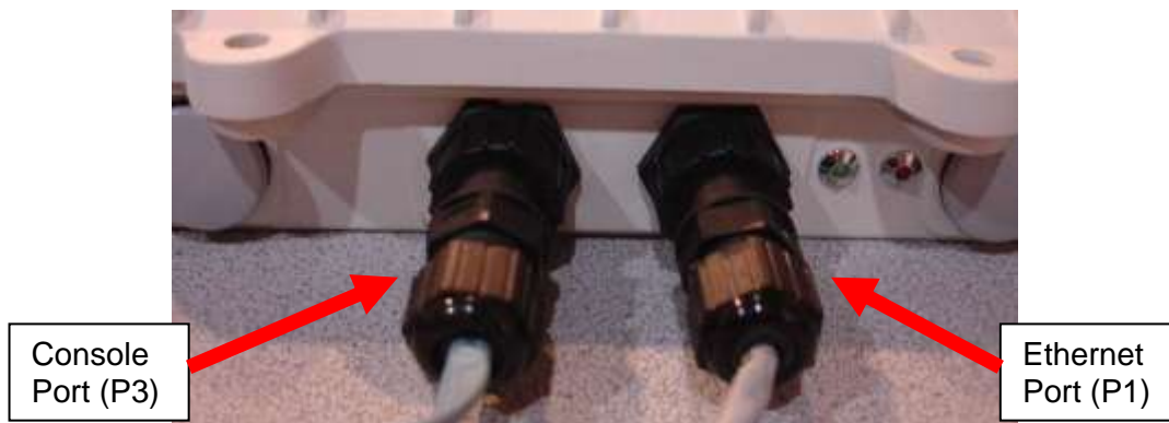
Figure 6: The FMG-3's front connectors
