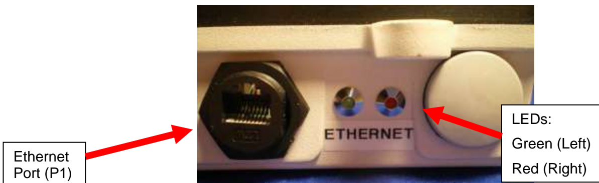
Figure 4: Close-up of P1 and the FMG-3's LEDs
