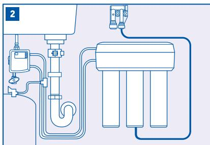
Connect the drain line coming from the RO system to the small connection of the air gap device.
