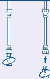
Disconnect the cold water line from the cold water shut-off valve.
