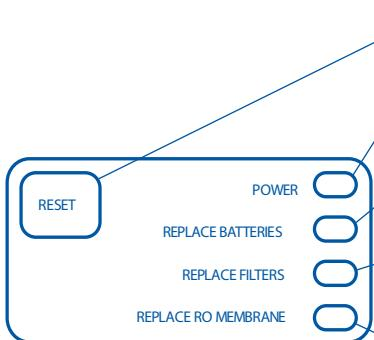
Reset button for filter capacity.
