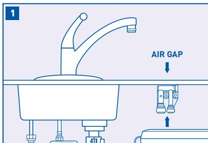
Mount the air gap device as near to counter top as possible and in a vertical orientation.
