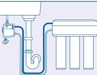
Connect the outlet on the RO/Filter system to the white port marked "RO/Filter <." Wet the end of the plastic tubing with water and push it into the quick connect fitting adapter approximately 5/8" until it stops.
