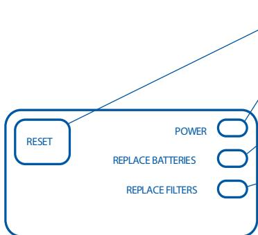
Reset button for filter capacity.
