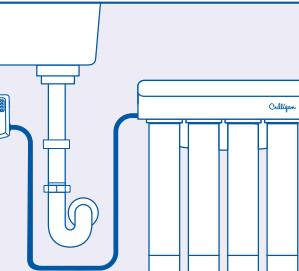
Connect the inlet on the RO/Filter system to the port marked "RO/Filter >." Wet the end of the plastic tubing with water and push it into the quick connect fitting adapter approximately 5/8" until it stops.
