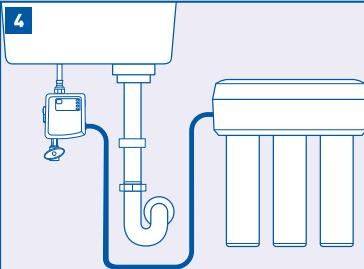
Connect the inlet on the RO/Filter system to the blue port marked "RO/Filter >." Wet the end of the plastic tubing with water and push it into the quick connect fitting adapter approximately 5/8" until it stops.
