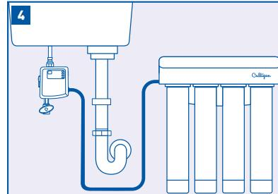
Connect the inlet on the RO/Filter system to the port marked "RO/Filter >." Wet the end of the plastic tubing with water and push it into the quick connect fitting adapter approximately 5/8" until it stops.
