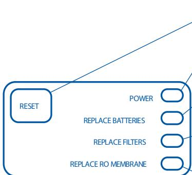
Reset button for filter capacity.
