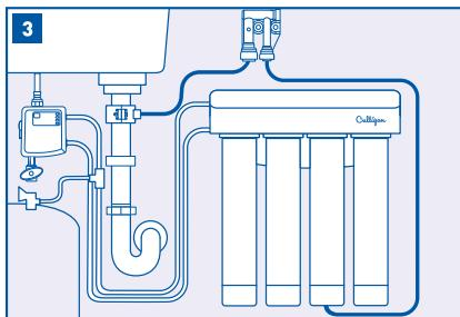
Connect the large fitting of the air gap device to the connection on the drain plumbing.
