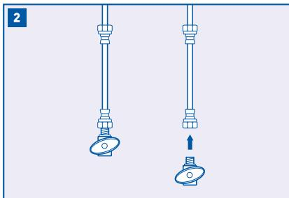
Disconnect the cold water line from the cold water shut-off valve.
