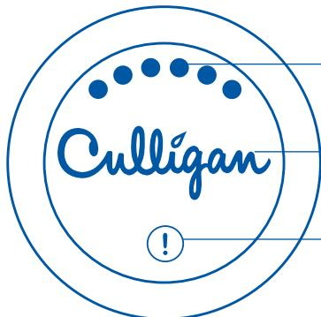
Filter Capacity Lights: Shows from 1-6 lights depending on filter capacity remaining, 6 lights = >80% and 1 light = <10%.
