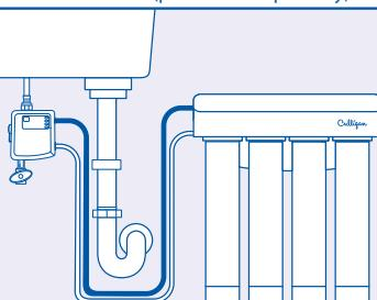
Connect the outlet on the RO/Filter system to the port marked "RO/Filter <." Wet the end of the plastic tubing with water and push it into the quick connect fitting adapter approximately 5/8" until it stops.
