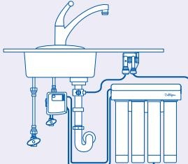
Turn on the cold water supply and check for leaks. If it leaks, refer to troubleshooting.
