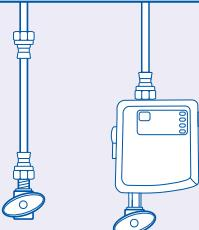
Tighten the control box to the cold water shut-off valve as shown. Tighten the lower end of cold water line onto the top of the control box.
