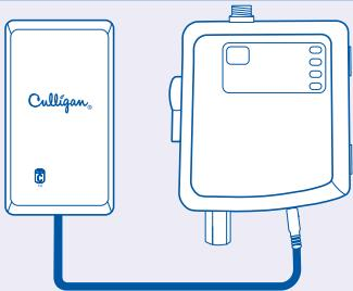
Install four C batteries (not included) into the battery box and plug into the jack on the bottom of the control box.
