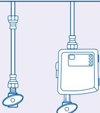
Tighten the control box to the cold water shut-off valve as shown. Tighten the lower end of cold water line onto the top of the control box.
