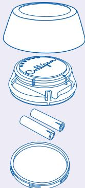
Install two AAA batteries (not included) into the remote button.
