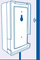
Use the provided screw to hang the battery box on the side of the cabinet.
