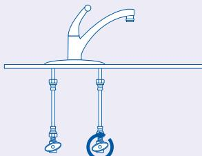
Turn off cold water shut-off valve then turn on the kitchen faucet and allow all water to drain from line.
