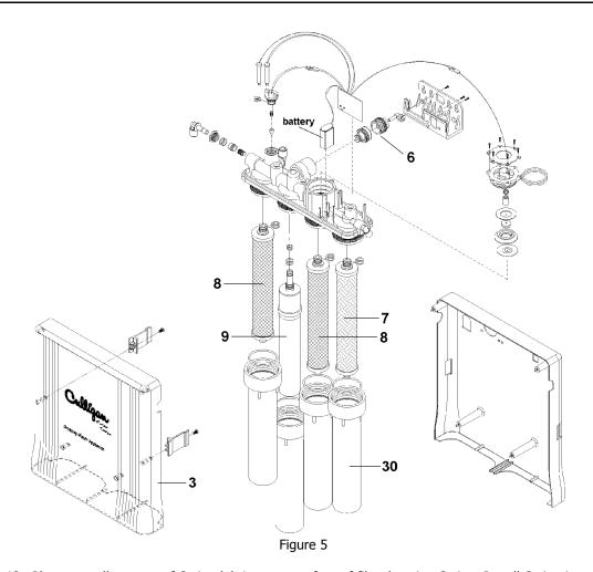
12. Place a small amount of O-ring lubricant on surface of filter housing O-ring. Install O-ring into housing.
