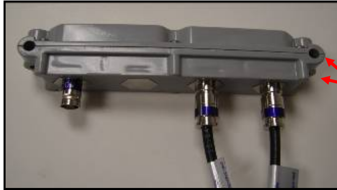
Figure 39 – Splitter mounting holes
