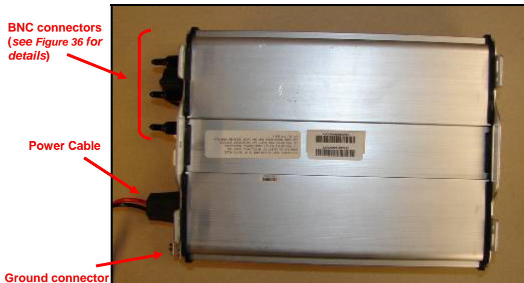
Figure 34 – CURRENT Bridge Nomenclature (front view)
