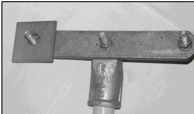
Figure 13 – 3" Square Washer Placement on T-strap
