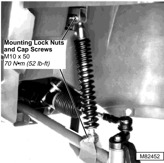
Standard Shock Absorber Mounting
