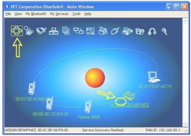
2.6 Single click one of the highlighted service icons, BlueSoleil will establish a Bluetooth connection to the remote device. The device icon changes to green color and a line appears between the red ball and the device icon.
