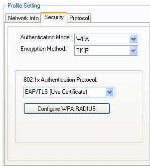
Figure 15: Security Tab—802.1x/WPA/WPA2 EAP/TLS Authentication
