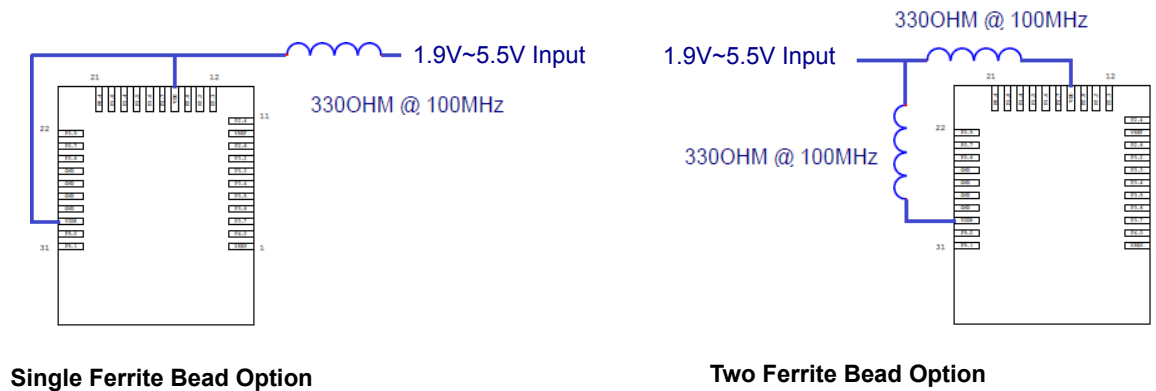
Figure 5. Recommended Host Schematic Options for a Single Supply Option
