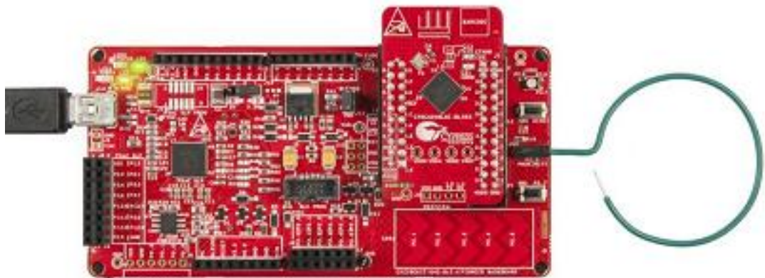
Figure 4-32. Proximity Sensor Connection on BLE Pioneer Kit with PSoC_4_BLE Module
