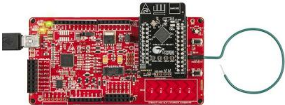
Figure 4-33. Proximity Sensor Connection on BLE Pioneer Kit with PSoC_BLE Module
