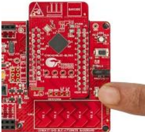
Figure 4-68. User Button on BLE Pioneer Kit with PSoC 4 BLE Module
