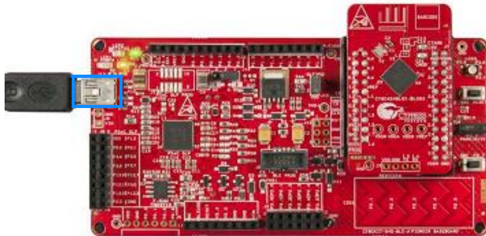
Figure 3-7. Connect USB Cable to J13
