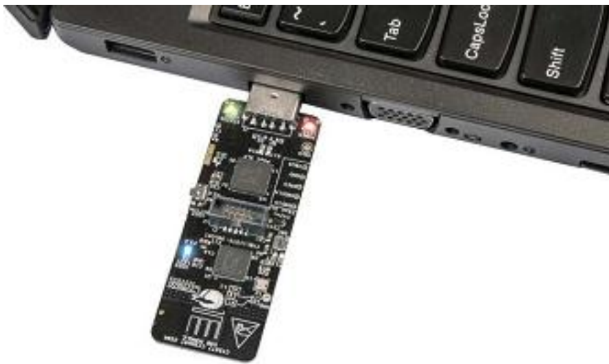
Figure 4-55. Connect BLE Dongle to USB Port
