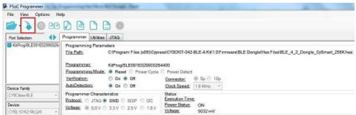
Figure 3-16. Programming Hex File to Dongle
