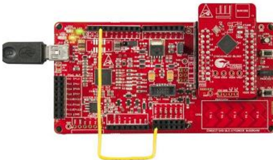
Figure 4-61. VREF (J3) and P3.0 (J2) Connectors on BLE Pioneer Kit with PSoC 4 BLE Module
