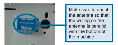
Attach the antenna cable to the DWL-AG520 by gently pushing it into the on-board connector.
