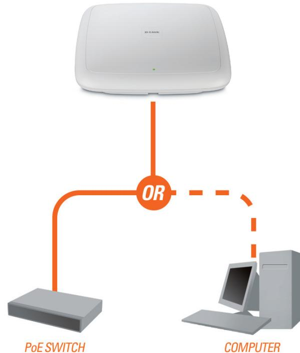
Connect one end of an Ethernet cable (included with your access point) to the LAN port on the DAP-2320L and the other end of the Ethernet cable to either your computer or to your PoE switch. The AP can be powered on by a PoE switch or by the power adapter shipped with the AP.
