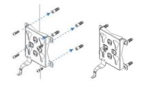
Securely mount the base to the wall using wall plug and wall screw.
