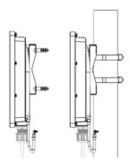
Attach the other end of the grounding wire to either the wall or pole mount. Ensure that the wall or pole mount is connected to an electrical ground.
