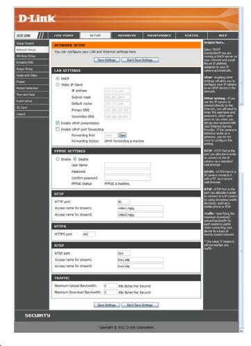
Maximum Upload/Download Specifying the maximum download/upload bandwidth Bandwidth: for each socket can be useful when connecting your device to a busy or heavily loaded network. Entering a value of '0' indicates that the camera should not monitor bandwidth. Specifying other values will limit the camera's transfer speed to the specified number of kilobytes per second.
