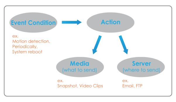
To start plotting an event, it is suggested to configure server and media columns first so that the network camera will know what action shall be performed when a trigger is activated.
