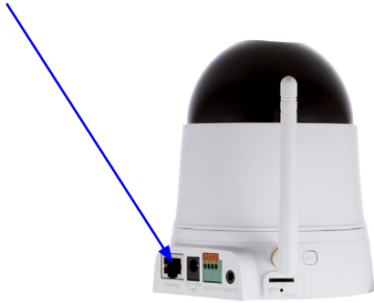
Connecting to a router
