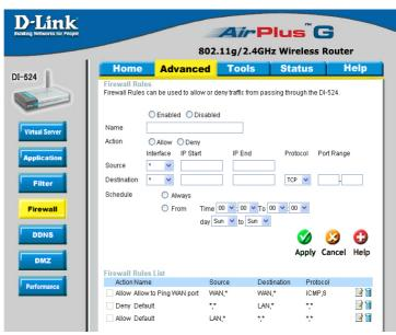
**Step 5** Select **LAN** as the **Destination** and enter the IP Address of the computer on your local network that you want to allow the incoming service to. This will not work with a range of IP Addresses.
