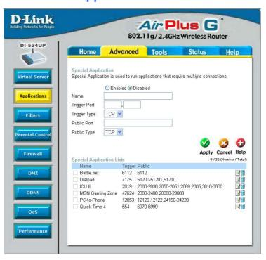
Applications Click the appropriate corresponding radio button to enable or disable the Applications feature.
