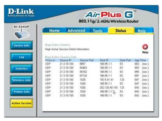
Sub-divided again, this window displays more detailed information on the TCP/UDP actions taken by the specific IP address, as stated below.
