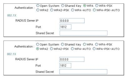
RADIUS Server IP Enter the IP address of the remote RADIUS server through which you will be authenticated.
