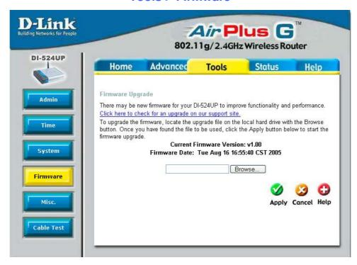
You can upgrade the firmware of the Router here. Make sure the firmware you want to use is on the local hard drive of the computer. Click on **Browse** to browse the local hard drive and locate the firmware to be used for the update. Please check the D-Link Support site for firmware updates at http://support.dlink.com. You can download firmware upgrades to your hard drive from the D-Link support site.
