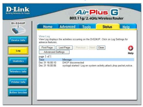
The Router keeps a running log of events and activities occurring on the Router. If the device is rebooted, the logs are automatically cleared. You may save the log files under **Log Settings**.
