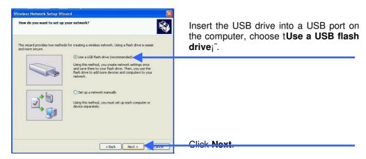
The settings will the automatically be uploaded to your USB flash drive. Once saved the user is to unplug the device, in the proper method, and then plug that USB flash drive into all devices that will be accessing the wireless LAN. Each device will upload the configurations automatically and be instantly accessible on the wireless LAN.
