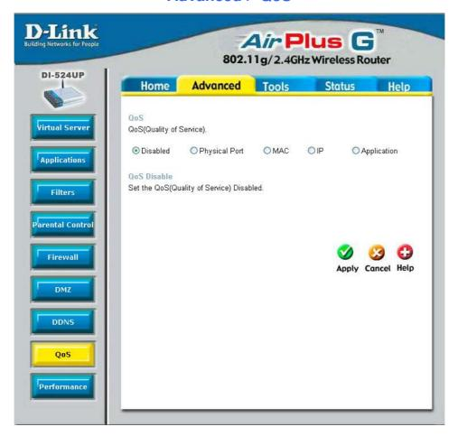
QoS or Quality of Service is used to allot bandwidth and priority from the router. To allot bandwidth per port on the router, click the appropriate **QoS** radio button and configure the parameters. QoS may be configured per **Physical Port**, **MAC address**, **IP address** or specified application. See the following explanation for more detailed information on each type of QoS setting.
