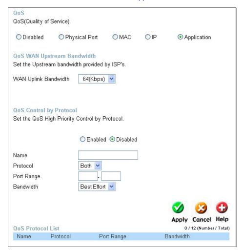
The user may also set QoS by specific protocol. To enable QoS per protocol, first click the **Application** radio button which will reveal the preceeding screen for the user to configure. Ensure that the bandwidth does not exceed the incoming bandwidth from the ISP or it will cause other devices on the LAN to slow down due to decreased bandwidth. Check with your ISP for more information on the bandwidth allotted to your account.
