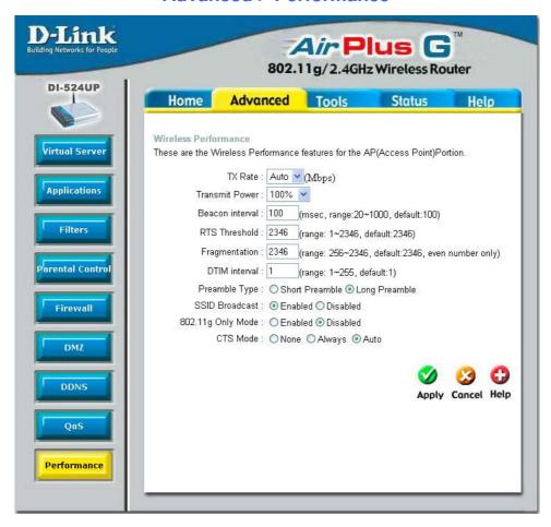
The **Performance** window is used to configure settings for the Access Point feature of this device. Configuring these settings may increase the performance of your router but if you are not familiar with networking devices and protocols, this section should be left at its default settings. Below is a list of the functions associated with the Access Point feature of the router. Click **Apply** when you have completed your changes.
