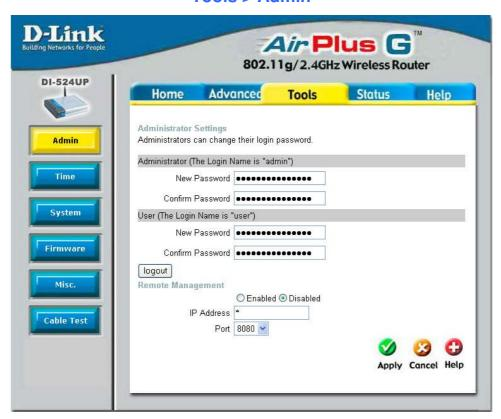
With this window, the DI-524UP administrator can change the system password. There are two accounts that can access the Broadband Routerifs We-Management interface. They are admin and user. Admin has read/write access while user has read-only access. User can only view the settings but cannot make any changes.
