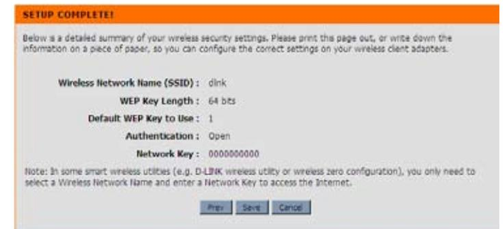
The Router will save your new settings and reboot. When it is finished after 1-2 minutes, the opening Wireless Setup window is displayed.
