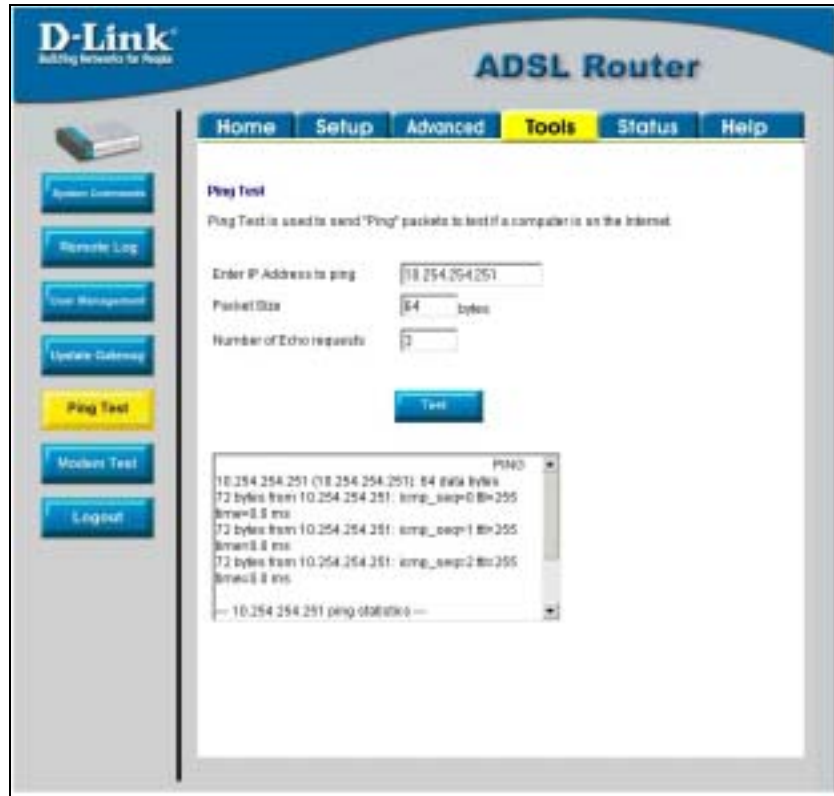
Figure 4-18. Tools – Ping Test window
