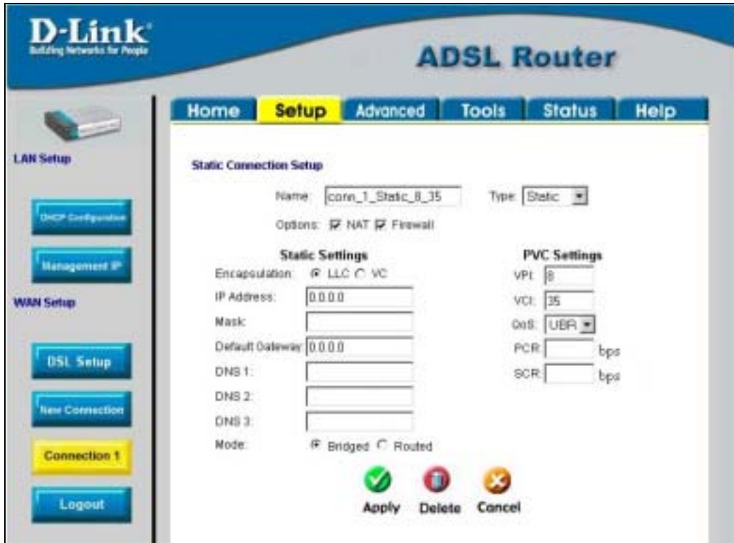
Figure 3-8. Setup – Configure Connection 1 for Static IP for the WAN
