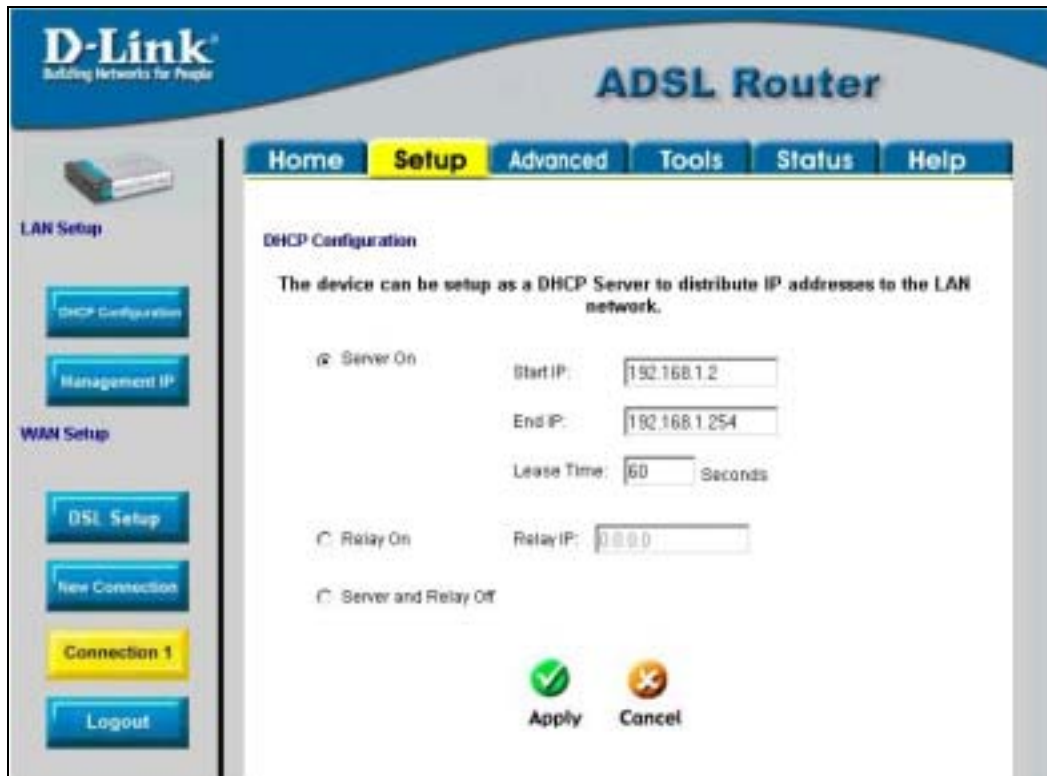
Figure 3- 13. Configure DHCP service for the LAN
