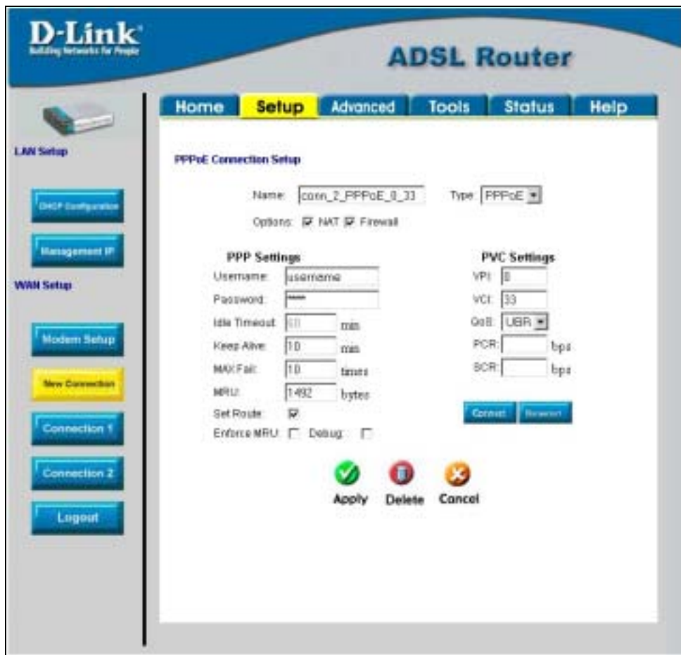
Figure 3- 11. Setup a New Connection – Connection 2
