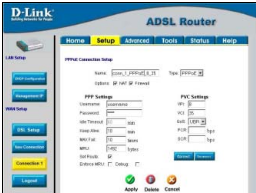
Figure 3-6. Setup – Configure Connection 1 for PPPoE
