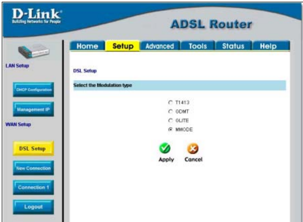
Figure 3-4. DSL Setup menu (change modulation type)
