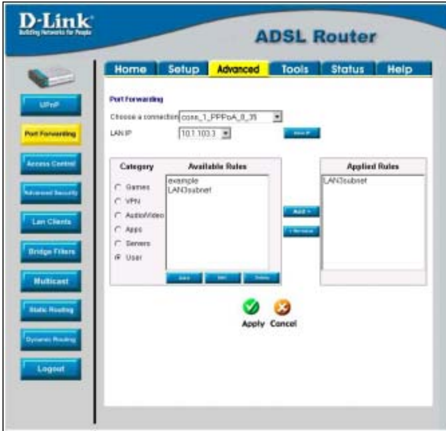
Figure 4- 5. Set up Custom Port Forwarding Rules
