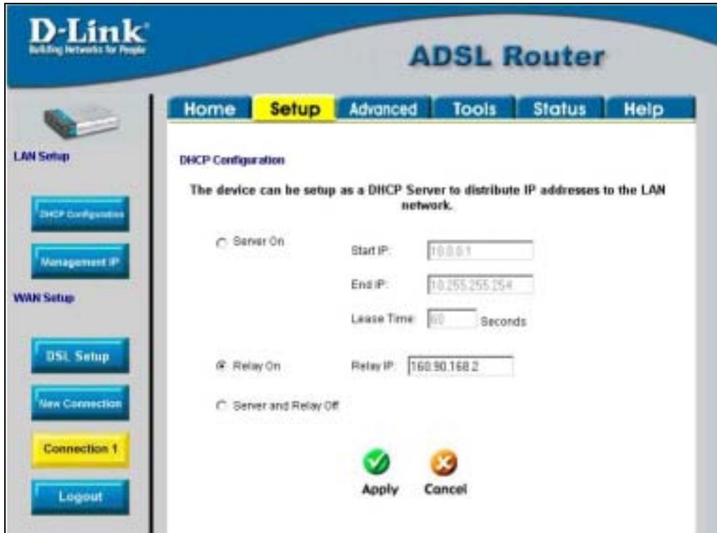
Figure 3- 14. Configure DHCP Relay Service
