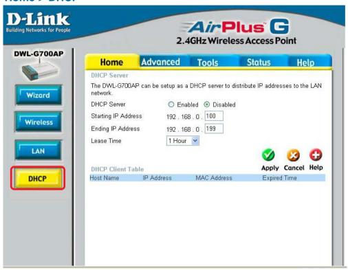
**DHCP Server:** Select **Enabled** or **Disabled**. Disabled is the default setting. If you want to use the DWL-G700AP as a DHCP server, to automatically assign dynamic IP addresses on the network, you will select Enabled.
