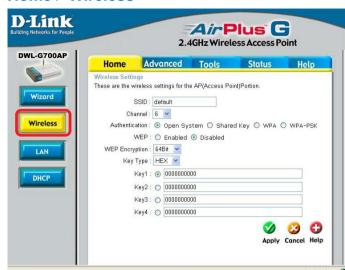
**SSID:** (Service Set Identifier) Default is the default setting. The SSID is a unique name that identifies a network. All devices on a network must share the same SSID name in order to communicate on the network. If you choose to change the SSID from the default setting, input your new SSID name in this field.
