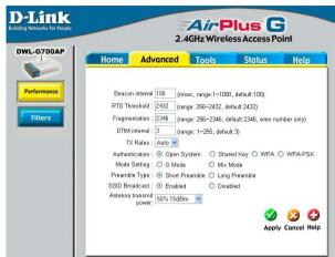
of 2,346. If you experience a high packet error rate, you may slightly increase your fragmentation threshold within the value range of 256 to 2,346. Setting the fragmentation threshold too low may result in poor performance.
