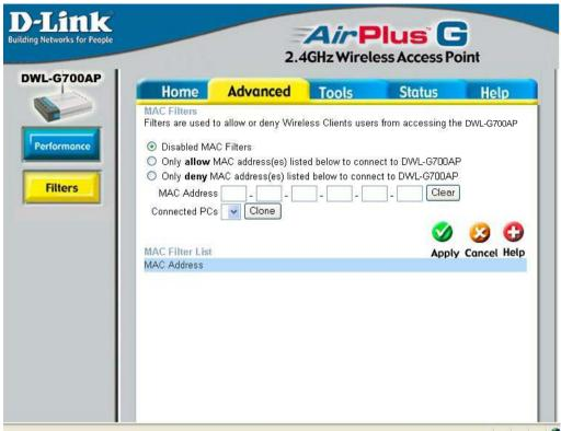
Use MAC Filters to allow or deny wireless clients, by their MAC addresses, from accessing the DWL-G700AP. You can manually add a MAC address or select the MAC address from the list of clients that are currently connected to the router (Connected PCs). The default setting is Disabled MAC Filters.
