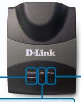
WLAN LED: A solid light indicates that the wireless segment is ready. This LED blinks during wireless data transmission.
