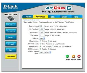
a high packet error rate, you may slightly increase your fragmentation threshold within the value range of 256 to 2346. Setting the fragmentation threshold too low may result in poor performance.
