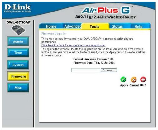
You can upgrade the firmware of the router here. Make sure the firmware you want to use is on the local hard drive of the computer. Please check the D-Link support site for firmware updates at http://support.dlink.com. You can download firmware upgrades to your hard drive from the D-Link support site. After you have downloaded the firmware upgrade to your hard drive, click **Browse** to browse the local hard drive and locate the firmware to be used for the update.
