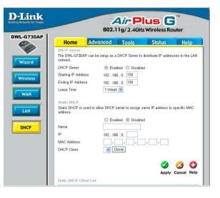
computer. You must specify the starting and ending address of the IP address pool.
