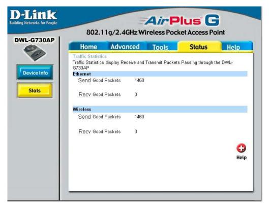
This screen displays theTraffic Statistics. Here you can view the amount of packets that pass through the DWL-G730AP on both the Ethernet and the wireless networks. The traffic counter will reset if the device is rebooted.
