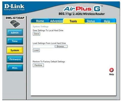
The current system settings can be saved as a file onto the local hard drive. To reload a system settings file, click on **Browse** to browse the local hard drive and locate the system file to be used.
