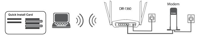
If you are configuring the DIR-1360 from a PC with a wired Ethernet connection, plug one end of an Ethernet cable into the port labeled 1 on the back of the router, and the other end into the Ethernet port on your computer.
