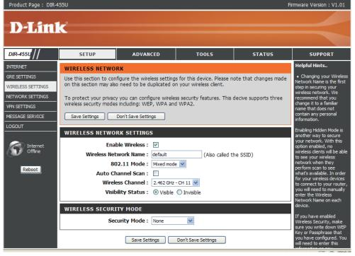
Auto Channel Scan: A wireless network uses specific channels in the wireless spectrum to handle communication between clients. Some channels in your area may experience interference from other electronic devices. Choose the clearest channel to help optimize the performance and coverage of your wireless network.
